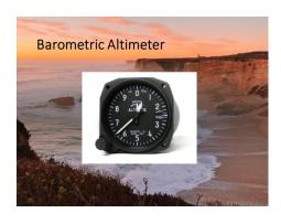
Now, a barometric altimeter uses an atmospheric pressure reading to determine altitude. I have installed or replaced them during my career in Coast Guard Aviation. At the beginning of each flight, the pilots set it for that day's sea-level
